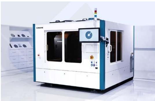
Picture 2: ICJet series — Industrial production equipment for frontend and backend semiconductor processes, supporting wafer and panel substrates.
